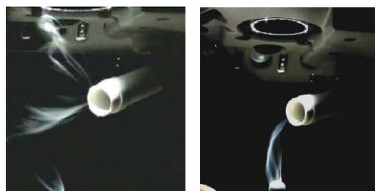
**Figure 2a:** Smoke generation demonstrating random vortices of plume propelled towards last optic in a turbulent distal evacuator.
